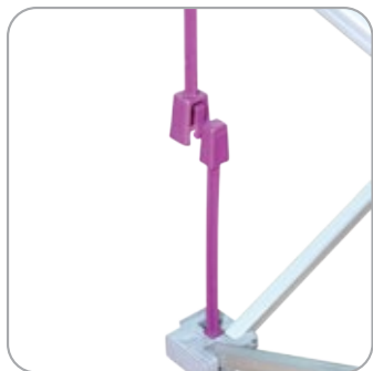
When setting up, ensure that the arms are aligned. If not, the arms will snap when pressure is applied.
